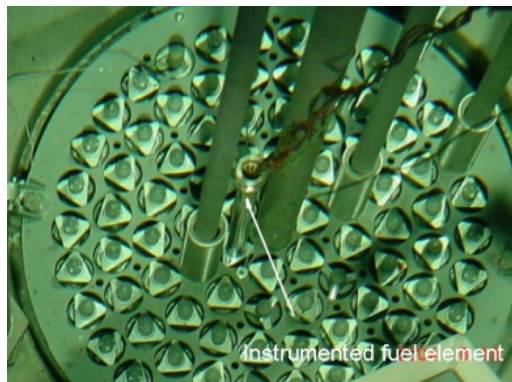
Fig. 19. Core upper view with the instrumented fuel element (Zacarias Mesquita and Cesar Rezende, 2010)
